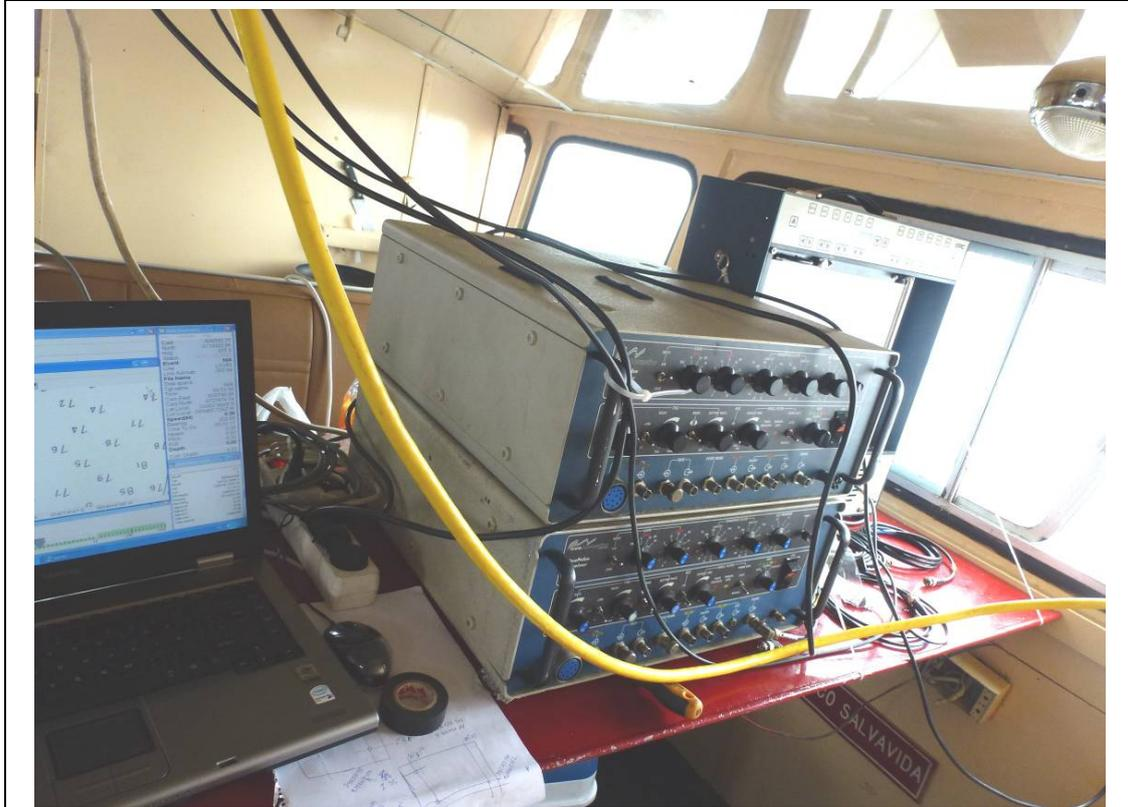
Receiver, Transceiver y EPC del Sistema Uniboom
